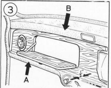
Open cubby lid and position panel into the car by resting the bottom edge on the parcel shelf rail. (a) Press the top edge back firmly to rest against the ledge on underside of the screen rail (b) the end to fit tight up to the instrument panel surround. Ensure that the bottom edge of the polished panel is approx. 1/2" parallel from the front edge of the parcel shelf rail.
