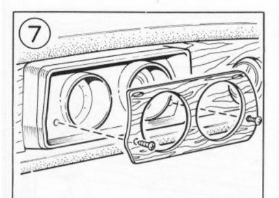
Position polished panel over instruments and drill and fix using 1/16" dia. drill and two 7/8" x No. 4 screws. TAKE CARE NOT TO OVER TIGHTEN SCREWS.
