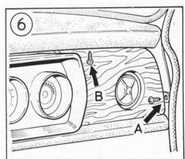
Position and fix short polished panel on drivers side in a similar manner as instructions "5". First fix bracket (a) and then (b). In each case press the panel firmly back but ensure that the bottom edge is approx. 1/2" from the front edge of the parcel shelf rail.
