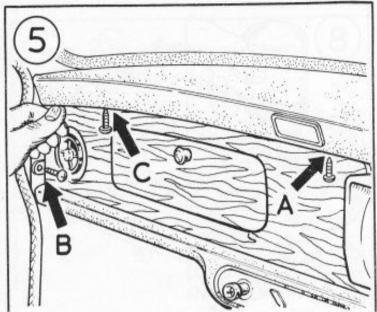
Press the top corner of panel (nearest instrument panel) firmly back and drill up through the bracket.
