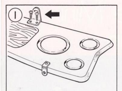
Line up holes in large angle bracket with pilot holes drilled into back of board and assemble as illustrated using two 5/16"x No. 6 screws. Screw door pull into hole in face of cubby lid.
