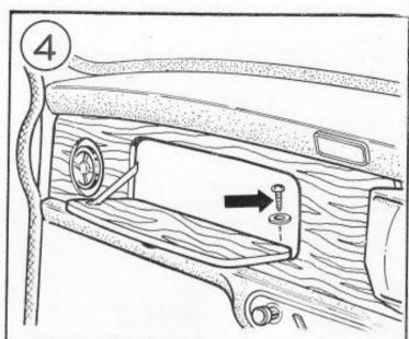
With the polished panel in position pierce the trimming through the hole in the large bracket. Remove the polished panel and using a 3/32" dia. drill, drill through the trimming and metal of the parcel shelf at the position marked. Replace the panel and fix using one 7/8" x No.4 self tapping screw and flat washer.
