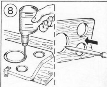
Provision is made for fitting extra gauges into polished wood panel (passengers side). Place panel polished face down on to a flat clean piece of wood. Use a 3/16" drill and holding it against the centre boss of wood, drill a circle of holes close together. Press the circle out from the polished side and use a half round file to clean it up to size. With the polished surface you file only one way. Do not draw the file back across polished edge otherwise chipping will occur.
